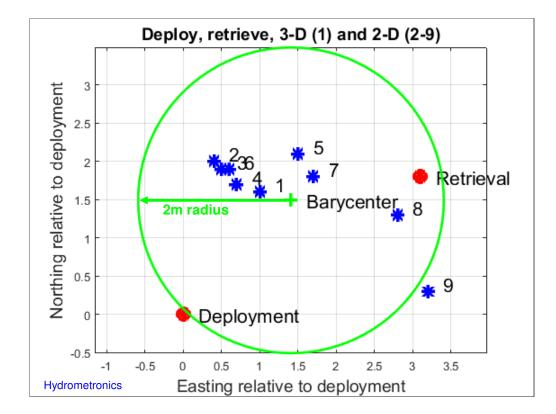
•In fact, if we plot the barycenter of all 9 first-break positions plus the USBL positions and draw a circle with a radius of 2 meters we capture almost all of it
