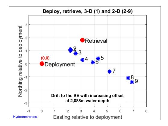
•This is a plot of the USBL deployment and retrieval positions in red relative to the deployment position, which is (0,0) in this plot
