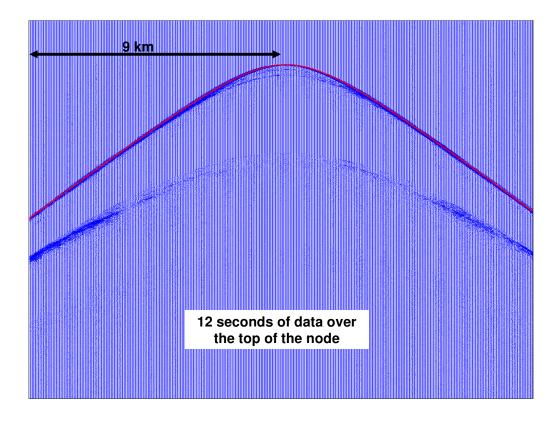
•Subsequent to the abstract another enhancement to the software was the plotting of seismic data with picks superimposed.
