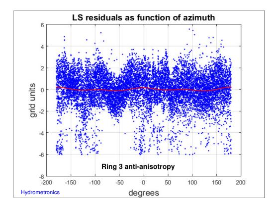
•After iteratively compensating for anisotropy the residual plot looks like this.
